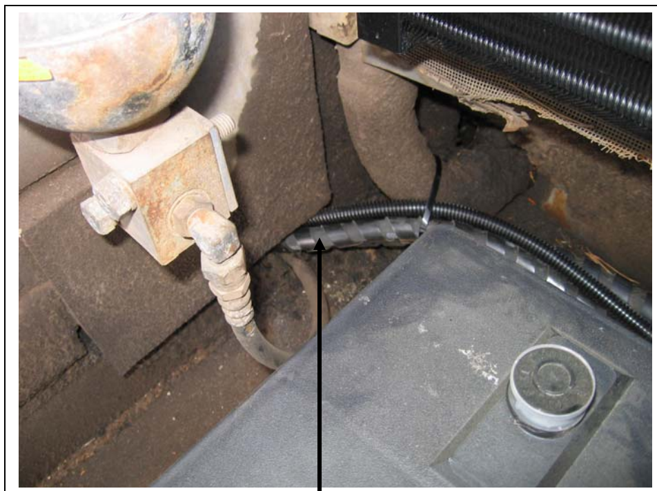
5/16" and 1/2" hose plus clutch wire running behind the batteries in the radiator compartment forward towards the evaporator in the cab.
